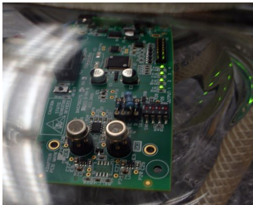
Figure 6: Two metal oxide ozone sensors (round, near the bottom) in the test chamber shown in Figure 9. Most of the volume of the sensor is the enclosure, and could be eliminated in a phone deployment. Photo by Virginia Teige.
