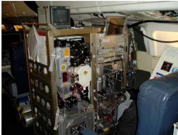
Figure 5: An extremely high precision spectroscopic NO 2 sensor mounted with an intake out the window of a DC-8. Photo courtesy of the Cohen Group at UC Berkeley.
