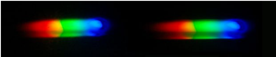
Figure 5: Spectral Data for 20 \mu\text{M} Methylene Blue. Left spectrum: I_0 . Right spectrum: I . Insets combined using Windows Paint. Line near the left end of the green part of the spectrum due to dirt on the grating. Note change in yellow part of spectrum due to MB absorption.
