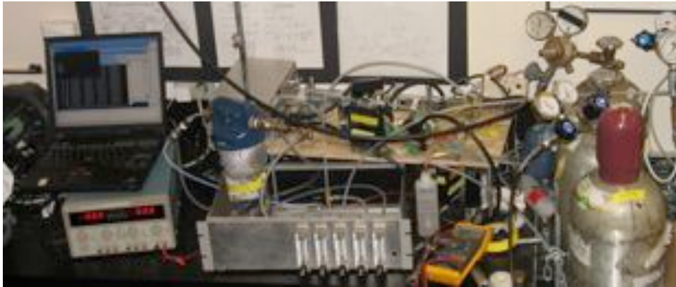
Figure 9: This setup has a small chamber that allows us to quickly change the concentration of poison gas in the chamber
