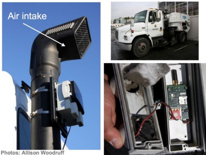
Figure 4a: A sensing device mounted on a street sweeper in San Francisco as part of the Intel CommonSense project.
