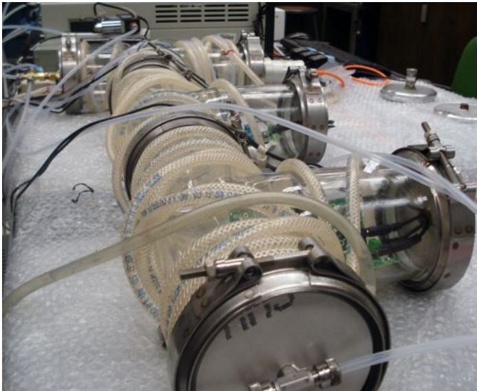
Figure 10: Another setup in our lab has a large chamber that allows us to test multiple large sensors simultaneously (Photo: Virginia Teige)
