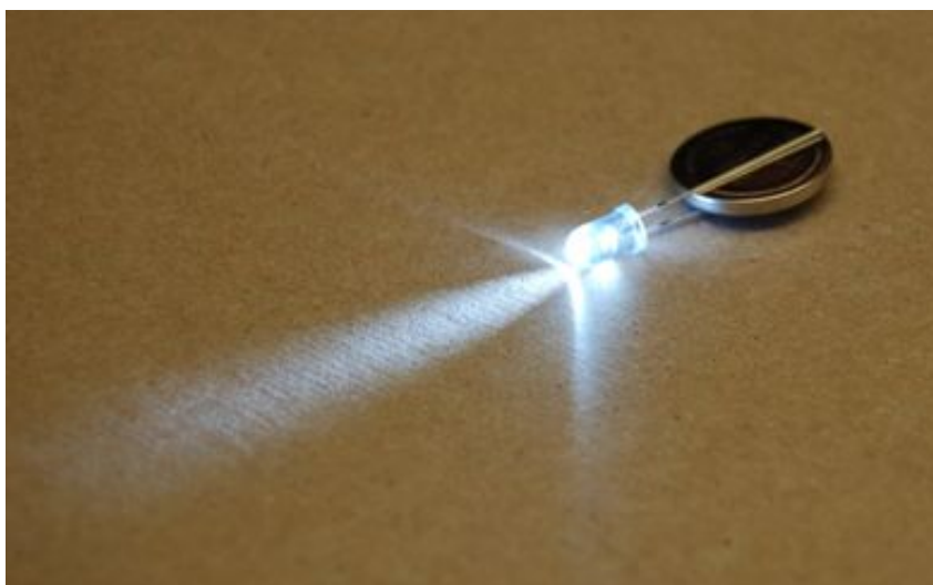
Figure 3: LED and Battery. LED diameter is 5 mm.
