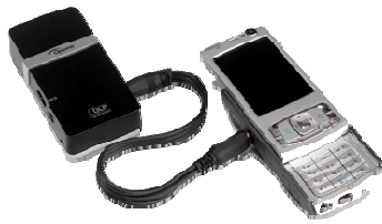
Figure 1. Camera phone (right) connected with pico projector (left) to emulate the functionality of a projection camera phone
