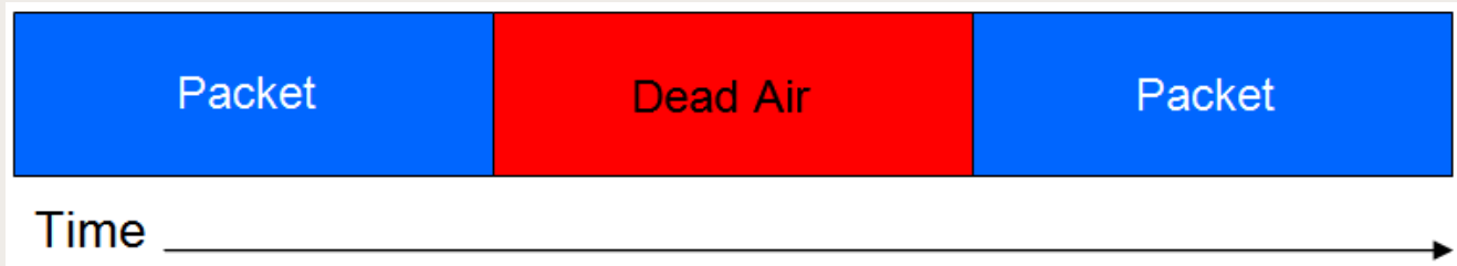
Figure 5: Carrier-sensing overhead in an IEEE 802.11n Contention System
