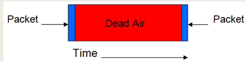
Figure 5: Carrier-sensing overhead in an IEEE 802.11n Contention System
